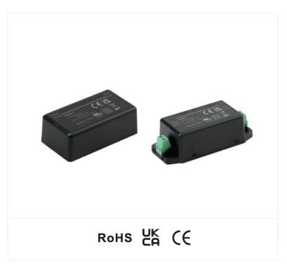
The 56YMR45-xy Series is a consistent and reliable 45W Encapsulated AC/DC PCB Mount Power Supply. Designed for use in applications such as commercial AV, broadcasting and control panels. This series is supplied with a Encapsulated input connection and supports input voltages of 100~277V AC 47-63Hz.
